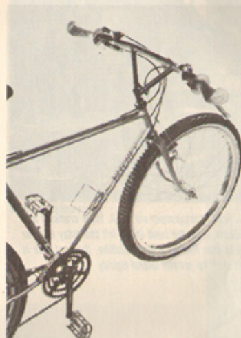
(Left) Tom Ritchey's MountainBike shows off its businesslike front end: motorcycle handgrips and brake levers, handy thumb shifters, and bullet-proof Bull Moose handlebars. Note also the second set of water bottle cage bosses on the seat tube and the black anodized T.A. triple crankset. Arne Ryason photo.
