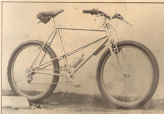
The Breezer: Chrome-moly hand made frame and forks, Phil Wood hubs and bottom bracket, motorcycle bars, Magura brake levers, KKT Lightning pedals, Campagnolo seat post and seat post clamp, Dia Compe cantilever brakes, and so on. 12 speeds. Cost is $1200.
