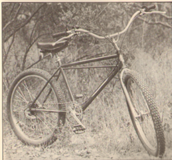
The Pro Cruiser: Chrome-moly frame, Tange forks, Shimano cranks, Messinger seat, Ukal aluminum rims, stainless steel spokes, Carlisle Nobby tires, etc. 5 speeds. Cost is $500.
