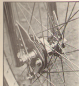
The Pro Cruiser runs Sturmey-Archer drum brakes front and rear.
